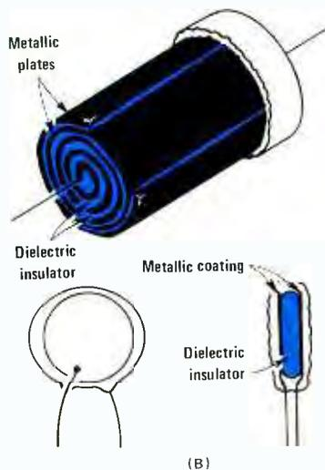
**Tubular capacitors (A) are made by rolling strips of paper or plastic insulation sandwiched between strips of metal foil. Ceramic disc capacitors (B) are made by coating the faces of a ceramic wafer with a metallic film.**
